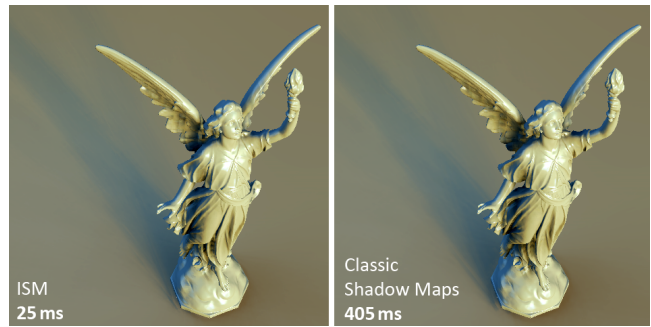
Figure 11: Depth map computation time for direct environment map illumination from 1024 VPLs using a model of 525 k faces with classic and imperfect shadow maps (256 × 256 and 8K points each).
