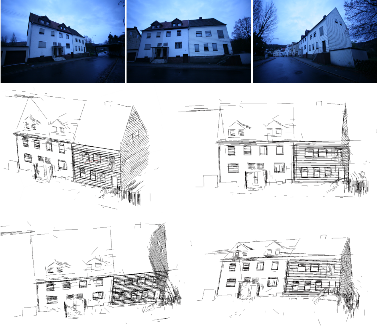
Figure 9. Street (real scene): Top: example images from the input sequence. Bottom: 3D line reconstruction with global connectivity constraints.
