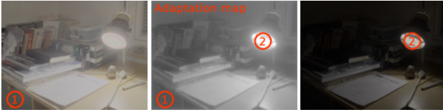
Figure 24: Two frames from a session with gaze-dependent tone mapping, in which an observer shifted their gaze from a dark to a bright image region. The map in the middle shows the spatial adaptation map predicted by our model. The circles with numbers show corresponding gaze positions.
