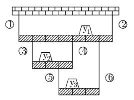
Cable 1 and 2 can bear a loading of 300 kg each, cable 3 and 4 only 100 kg each, and cable 5 and 6 only 50 kg each. Neglecting the weight of cables and planks, we are searching for the maximal allowed total weight  $y_1 + y_2 + y_3$ . Formulate this problem as a linear program.
