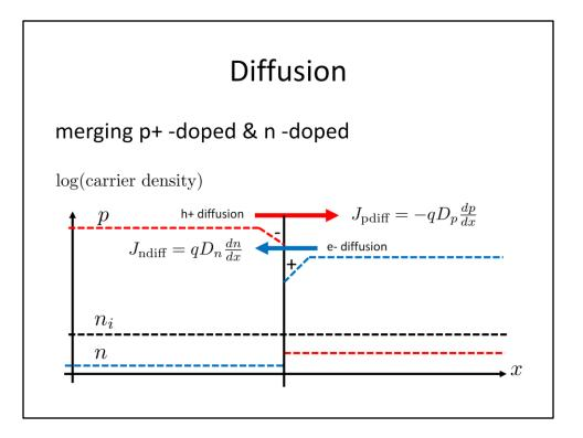
note: the donor and acceptor ions cannot move. They remain, but now are charged since e- is missing or extra (= hole missing)
