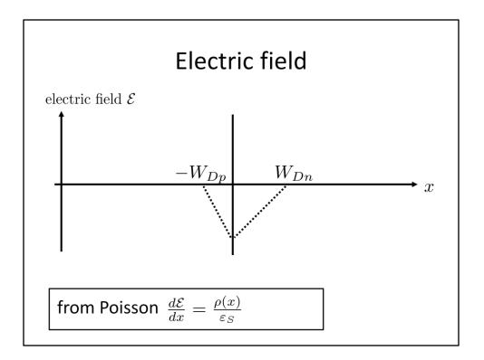
electric field induces a force on carriers. a positive carrier like a h+ is pushed to the left by a negative electric field.
