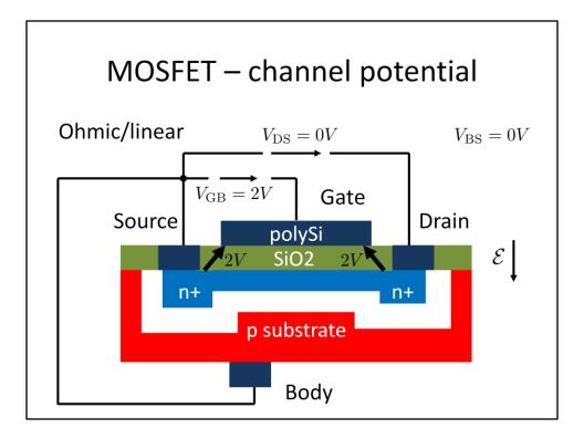
channel begin: 2V from channel point to gate. channel end: 2V from channel point to gate.
