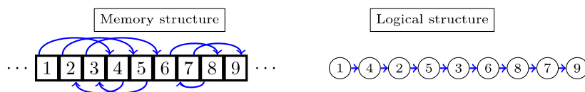
Figure 1.2: State after many insertion and deletion operations. There may also be “dead” cells which are currently not part of the list. These are not shown; we assume that these are taken care of every now and then to avoid wasting too much memory.
