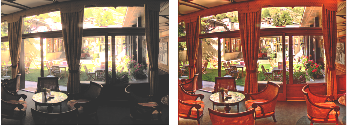
Figure 2. An example of artifacts due to the tone mapping of HDR images and HDR video sequences. Left: global tone mapping technique by Pattanaik et al. 11 preserves overall image contrast, but results in severe loss of details . Right: gradient-based technique of Fattal et al. 12 is able to reproduce virtually all the image details, at the cost of an overall contrast and contrast reversals (i.e. halo artifacts).
