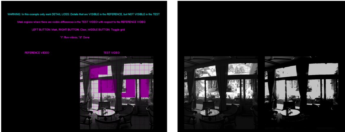
Figure 4. The experiment was performed through a graphical user interface on the HDR display. Subjects were shown reference and test videos side by side in a randomized order (right), and were asked to mark the relevant image locations on a 16 \times 16 grid according to the instructions (left). The interface and messages were disabled while the videos were being shown. The interface allowed the subjects to watch the videos for an unlimited amount of iterations.
