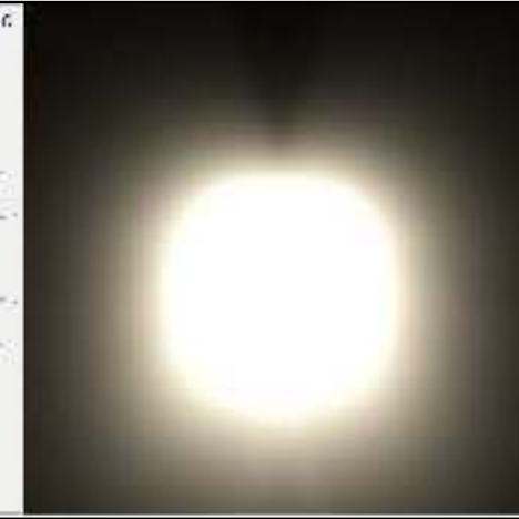
Emission goniometric diagram (far field photometry)
