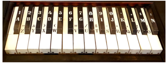
Figure 2: The Hughes-Phelps telegraph is a piano-based text entry device used in the 19th century by telegraph operators. Its design used a quasi-alphabetical ordering of letters to piano-like keys.
