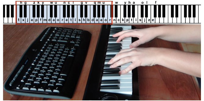
Figure 9: We redesign PianoText to be used on a 37 key piano, similar in size to a physical Qwerty keyboard. It shows the applicability of piano-based typing in a regular working environment.
