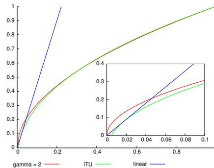
**Figure 7:** Comparison of the gamma power function usually used in computer graphics with the ITU-R BT.709 transfer function. The essential difference is the less drastic mapping of dark pixels in the ITU-R BT.709 function.
