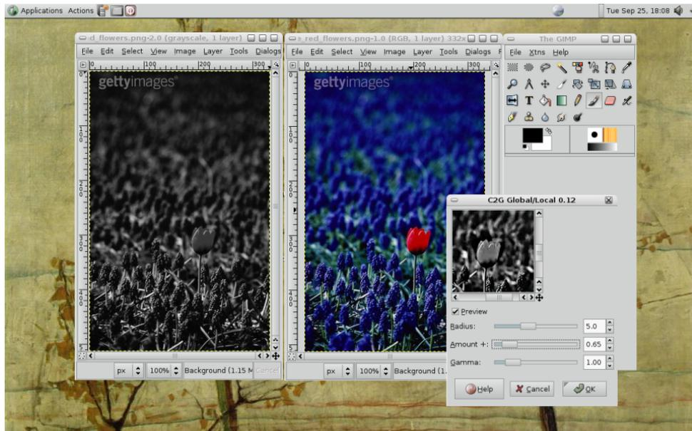
**Figure 16:** For quick testing, we implemented a single-scale version of our approach as a Gimp plug-in, with an adjustable filter size.
