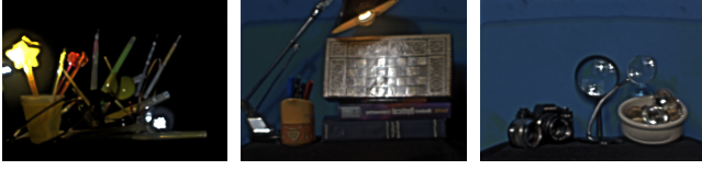
Figure 8: Tone-mapped results of three example scenes captured with our high dynamic range setup. The maximum dynamic range is about 18 f-stops.
