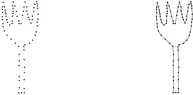
Figure 2: The left hand side shows a point set. The right hand side shows the optimum Traveling Salesman tour through this set of points. It is obtained as a solution of the sub-tour LP.
