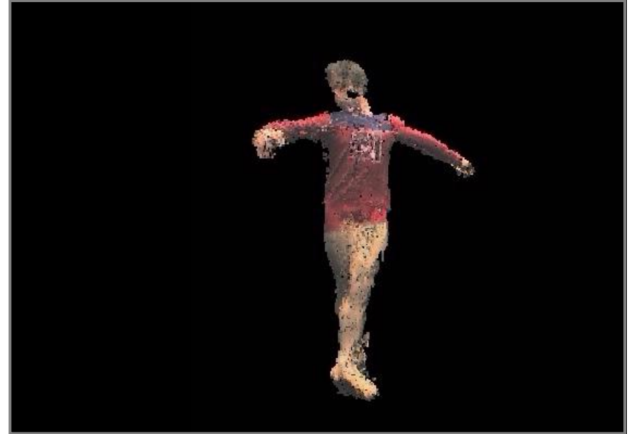
multi view matching (6 cameras) (photo-consistent space carving)
