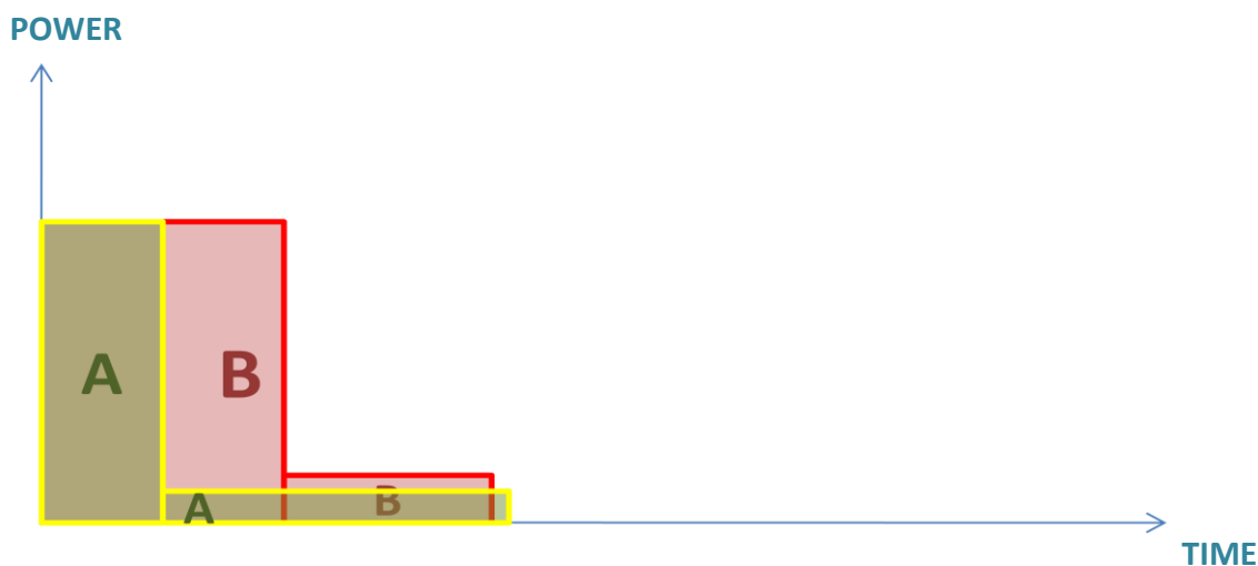
Figure 1: The figure shows two plans A and B for the same query. Plan A is less CPU bound but a little more I/O bound so its performance is a little bit better than that of plan B even though it has so much less CPU usage. As we know that the power usage of HDD is negligible compared with CPU power usage, plan B has more power and energy consumption than plan A.
