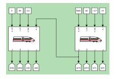
Minimal admissible distance d between two successive trains equals braking distance  $d_b$  of the second train plus a safety distance S.
