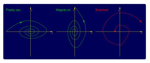
Interaction of continuous dynamics and discrete mode switch destroys global convergence!
