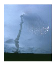
« On 4 June 1996, the maiden flight of the Ariane 5 launcher ended in a failure. Only about 40 seconds after initiation of the flight sequence, at an altitude of about 3700 m, the launcher veered off its flight path, broke up and exploded. »
