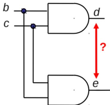
Parts of the miter which are relevant for the proof of  $d \equiv e$
