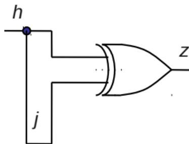
Parts of the miter which are relevant for the proof of  $z = 0$
