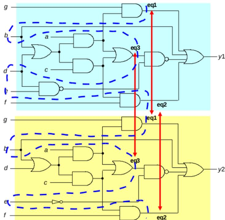
Cut the circuits at the internal equivalent signals
