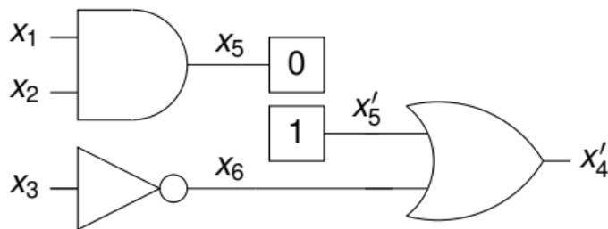
(b) Faulty circuit, s@1-error at  $x_5$
