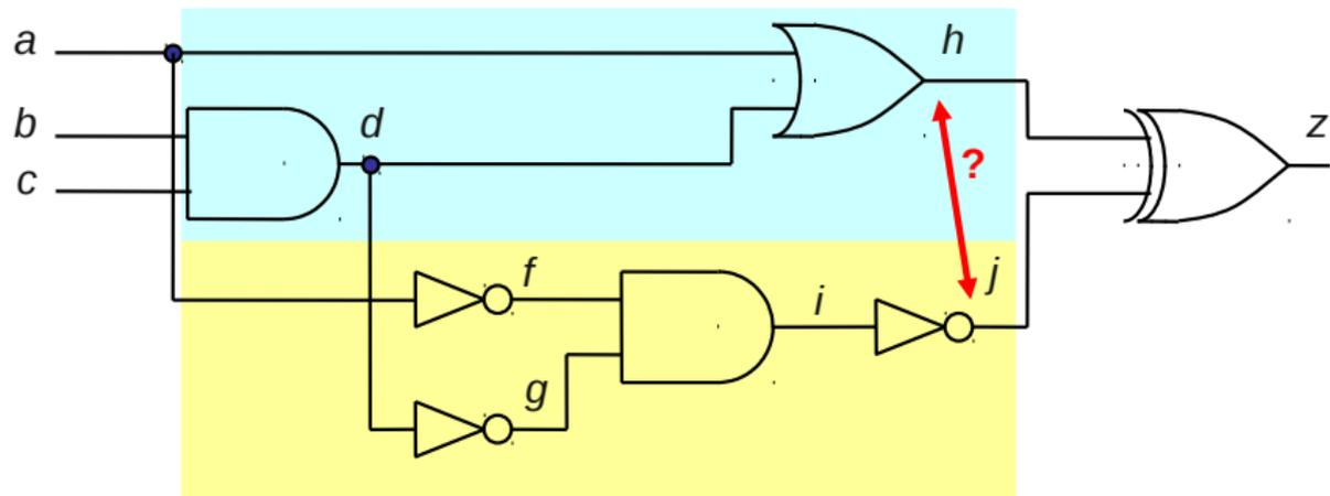
Are the internal signals  $h$  and  $j$  equivalent?
