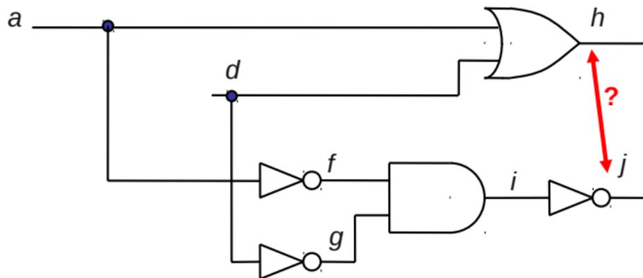
Parts of the miter which are relevant for the proof of  $h \equiv j$
