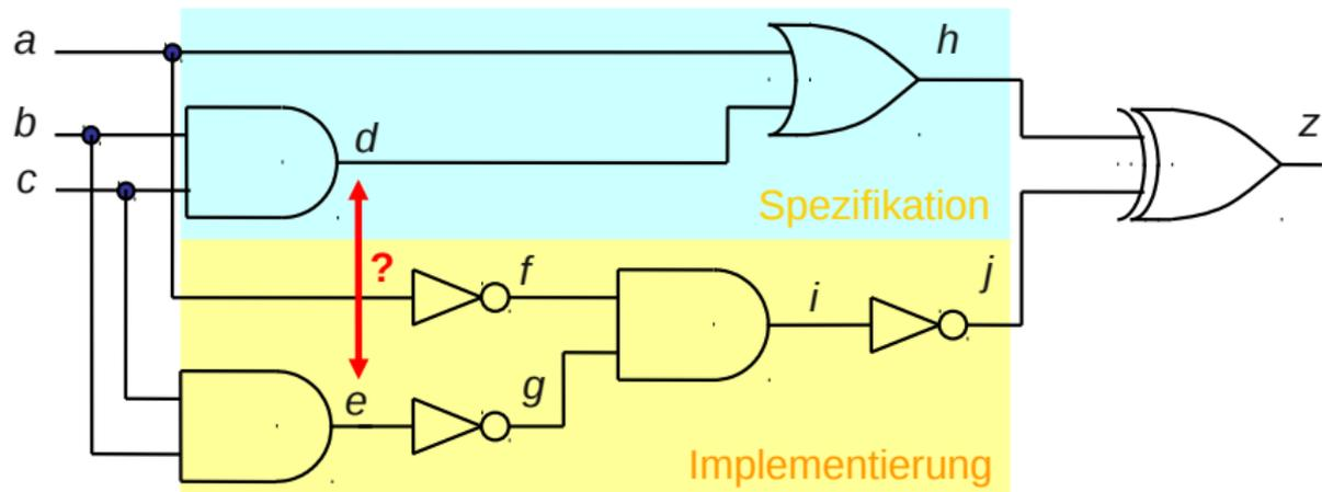
Are the internal signals  $d$  and  $e$  equivalent?
