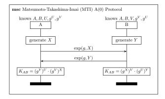
Message exchange as in basic DH; protocol combines long-term and ephemeral DH keys to authenticate exchanged DH public keys.
