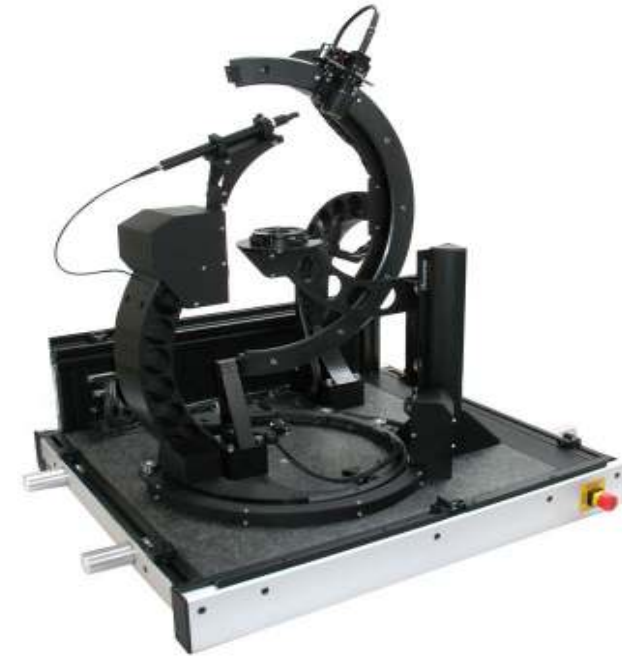
Gantry for BRDF acquisition Lightec company (France)
